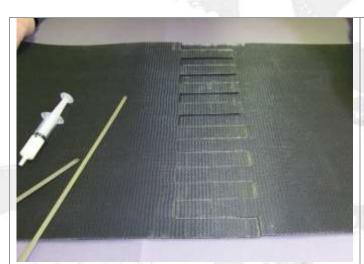
Then fit quickly the fingers of joint together by two ends. (The lubricant must not dry).
